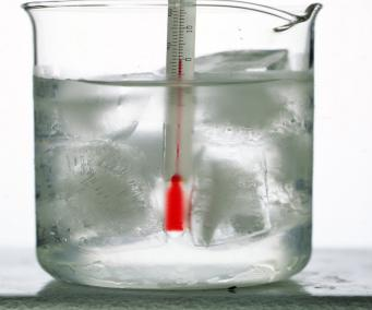
When we measure melting point the tip of thermometer must be placed in water enclosed between ice particles.
